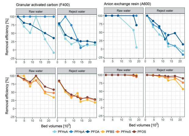
Fig. 2 Removal efficiency [%] of frequently detected PFCAs (top) and PFSAs (bottom) for the evaluated granular activated carbon material (F400, left) and anion exchange resin (A600, right) depending on bed volumes treated. Treatment of both raw water and water rejected by a NF270 membrane was evaluated. Please note that lines are solely added to guide the eye, and do not represent a model.
