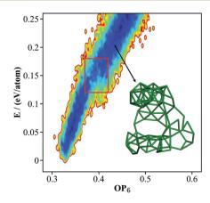
Fig. 3 The contour map (E against OP<sub>6</sub>, also see Fig. 1 caption for explanation) for the  $\beta$ -B minima from the SSW global optimization using the boron NN PES. The red box indicates the boundary above which the B<sub>28</sub> cages start to melt. The inset shows a typical structure with broken B<sub>28</sub> cages.
