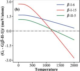
**Fig. 6** The phonon density of states (a) and the relative free energies (b) for the key configurations,  $\beta$ -I-6,  $\beta$ -I-15,  $\beta$ -II-5 and  $\beta$ -II-1. The relative free energy ( $G_i$  in eqn (13)) is with respect to that of  $\beta$ -II-1,  $G[\beta$ -II-1].
