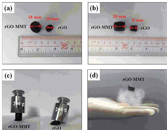
Fig. 1 The digital photos of rGO-MMT aerogel.
