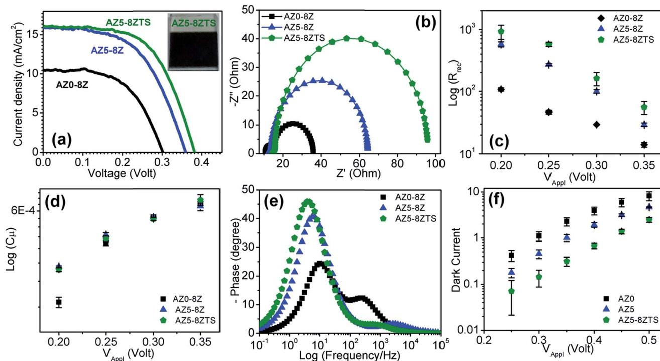
Fig. 4 (a)  $J$ - $V$  characteristics of the representative QDSSCs under 1 sun illumination. (Inset) Digital image of the AZ5-8ZTS photoanode. (b) Nyquist plot of the QDSSCs at  $-0.35$  V forward bias under dark conditions. Plots of the (c) recombination resistance and (d) chemical capacitance of the QDSSCs with applied potential. (e) Bode plots of the QDSSCs. (f) Variation of dark current with applied potential in the log scale.
