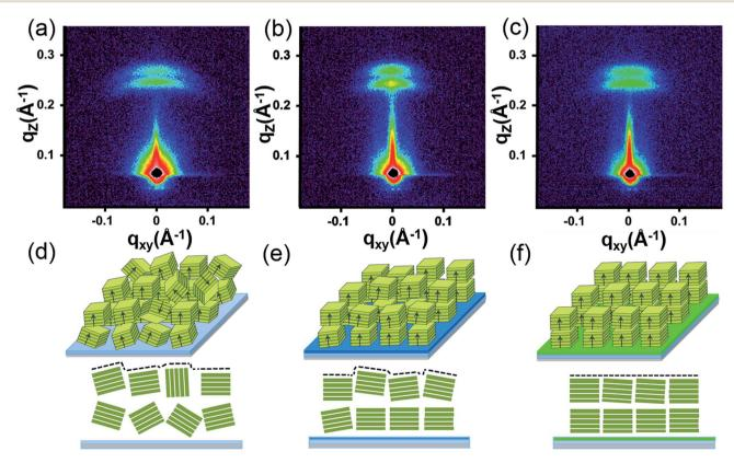
Fig. 4 (a)–(c) GISAXS pattern of SA-Bu evaporated on ITO, PPA–ITO and OPA–ITO substrates and (d)–(f) the proposed crystallite stacking models, respectively.
