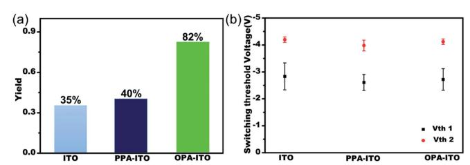
Fig. 3 (a) Ternary yield based on three types of substrates; (b) statistics for switching threshold voltages of both the  $V_{th}1$  state and  $V_{th}2$  state of ternary devices with error bars (variance).
