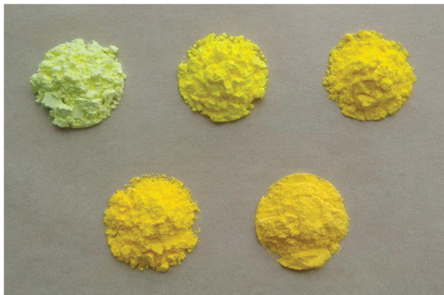
Fig. 12 Digital images of the as-prepared \text{Lu}_{2.95}\text{Ce}_{0.05}(\text{Al}_{2-x}\text{Mg}_x)(\text{Al}_{3-x}\text{Si}_x)\text{O}_{12} ( x = 0, 0.5, 1.0, 1.5, 2.0 ) phosphors under sunlight. The sample body-color turns from green to orange as x increases.
