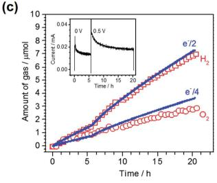
Fig. 2 Evolution of hydrogen/oxygen from the two-electrode system under visible light ( $\lambda$  > 420 nm) irradiation. (a) Pt/LTC/Au (3.5 cm²) – Pt wire under a bias of -0.9 V, (b) CoPi/LTC/Ti (4.3 cm²) – Pt wire under a bias of 0.8 V and (c) CoPi/LTC/Ti (4.5 cm²) – Pt/LTC/Au (2 cm²) under a bias of 0 and 0.5 V. The inset shows current–time curves recorded during the respective measurements.
