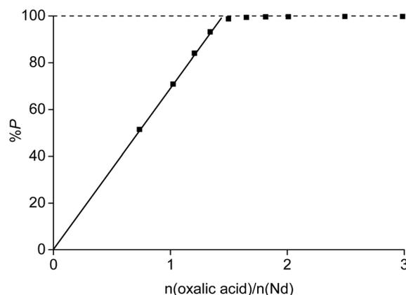
Fig. 13 Percentage precipitation (%P) as a function of the molar ratio of oxalic acid added to the solution over neodymium present in the aqueous phase  $n(\text{oxalic acid})/n(\text{Nd})$ . The aqueous phase contained 26.7 g  $\text{L}^{-1}$  neodymium and 3.5 M  $\text{NH}_4\text{Cl}$ .
