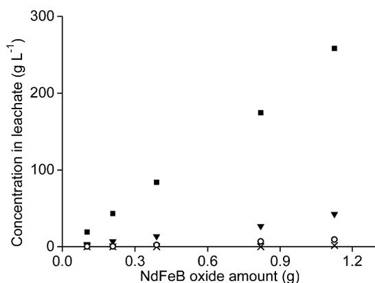
Fig. 9 Concentration of neodymium (■), dysprosium (▼), cobalt (○) and iron (×) in the leachate as a function of the amount of magnet oxide powder involved in leaching with 1 mL of aqueous phase. The  $n(\text{HCl})/n(\text{Ln})$  ratio was 3.5 and the pH after leaching between 3.3 and 2.76. The data point with the highest concentrations had a pH of 1.41. Standard deviation < 7.6%.
