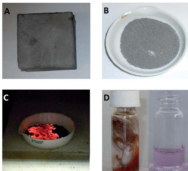
**Fig. 1** (A) The NdFeB magnet before crushing and milling, (B) NdFeB powder (<400 μm) before roasting, (C) roasting and powder fire at high temperatures and (D) the leachate colored pink-violet by neodymium (right) and the remaining orange/brown iron(III) hydroxide precipitate (left).
