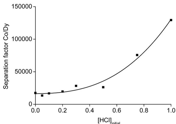
Fig. 12 The separation factors  $\alpha_{\text{Co,Dy}}$  between cobalt and dysprosium as a function of the initial HCl concentration of the aqueous phase. The aqueous phase contains 3.0 g  $\text{L}^{-1}$  cobalt, 25 g  $\text{L}^{-1}$  Dy and 3.5 M  $\text{NH}_4\text{Cl}$ . The organic phase was trihexyl(tetradecyl)phosphonium chloride mixed with the aqueous phase in a volume ratio of 1.
