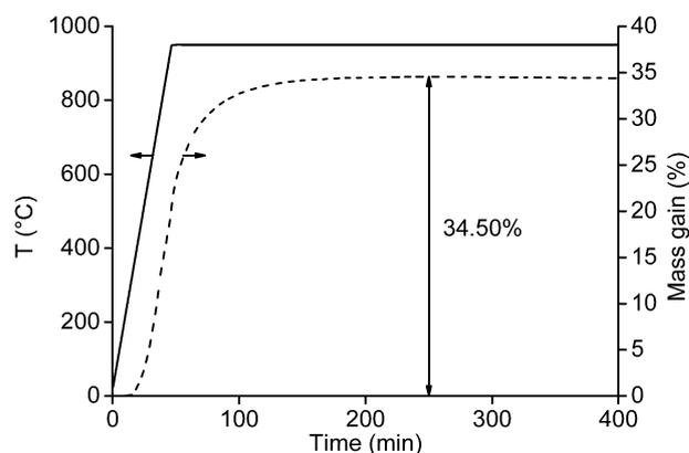
Fig. 2 Thermogravimetric analysis of the magnet powder <400 μm. The NdFeB magnet powder was first heated to 950 °C (heating rate: 20 °C min<sup>-1</sup>) and kept at this temperature for another 6 h. The temperature of the furnace is given by the solid line and the mass gain (%) by the dashed line.
