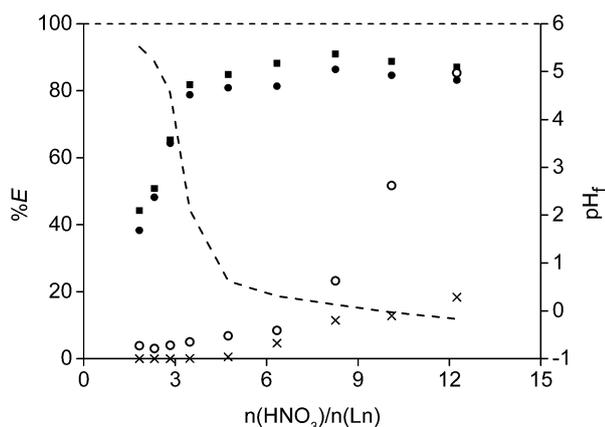
Fig. 6 Percentage extraction (%E) of neodymium (■), dysprosium (▼), cobalt (○) and iron (×) as a function of the molar ratio of  $HNO_3$  over the rare earths present in the roasted NdFeB magnet powder. The dashed line shows the measured final pH values ( $pH_f$ ) after the leaching experiments. Relative standard deviation < 6.9%.
