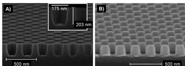
**Fig. 6** SEM images of (A) the hard silicon master with depth and width noted inset, and (B) the soft stamp cast obtained from photocuring the PMMS/TAC/BPDMA mixture. Reproduced by permission of WILEY-VCH from ref. 80: Campos *et al.*, *J. Adv. Mater.*, 2008, **20**, 3728–3733. DOI: 10.1002/adma.200800330.
