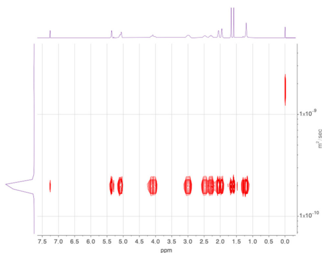
Fig. 6 DOSY NMR spectrum of polyester- block -polycarbonate formed from anhydride M4 , PO, and CO 2 (Table 2, entry 9) in CDCl 3 at 298 K. Data obtained from analysis of DOSY NMR spectrum: D = 1.97 \times 10^{-10}\text{ m}^2\text{ s}^{-1} .
