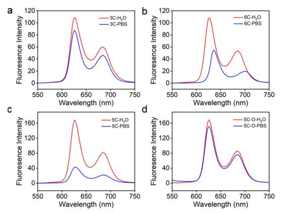
Fluorescence spectra of 3C (a), 6C (b), 5C (c), and 5C-O (d) in H<sub>2</sub>O (red) or PBS (blue)
