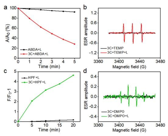
Fig. 5 (a) Decomposition rates of ABDA with or without the presence of 3C with increasing illumination time. (b) ESR signals of 3C to detect the generation of  ${}^{1}O_{2}$  after irradiation using TEMP as a spin trapper. (c) Fluorescence changes of HPF with or without the presence of 3C with increasing illumination time. (d) ESR signals of 3C to detect the generation of OH $^{*}$  using DMPO as a spin trapper.
