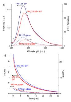
Fig. 6 (a) Fluorescence spectra of **Rh123** and **Rh123-2Br** on the glass and SIF surfaces; (b) the time-dependence of the DF ( $\lambda_{\rm reg} = 540$  nm) and phosphorescence ( $\lambda_{\rm reg} = 670$  nm) decay of **Rh123-2Br** on the glass and SIF surfaces.
