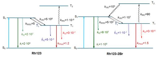
Fig. 5 The Jablonsky diagram of Rh123 and Rh123-2Br
