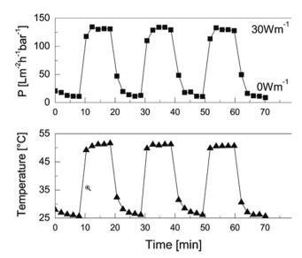
Fig. 6 The dead-end permeability (P) through a Si-C membrane with PVCL microgel coating was measured with heating cycles of 10 min with 30 W m<sup>-1</sup> of applied power. The permeability is increased due to the collapse of the microgel. Reproduced with permission from T. Lohaus, P. de Wit, M. Kather, D. Menne, N.E. Benes, A. Pich and M. Wessling, J. Membr. Sci., 2017, 539, 451.
