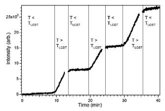
Fig. 9 Reversible switching capability of the pNIPAM grafted membrane Permeation of 77 kDa dextran over several heating-cooling cycles measured over time via fluorescence. At each gate opening, the dextran concentration increases resulting in a higher intensity. Reprinted with permission from Lokuge, I. et al. (2007), 23(1), 305-311. Copyright 2007 American Chemical Society
