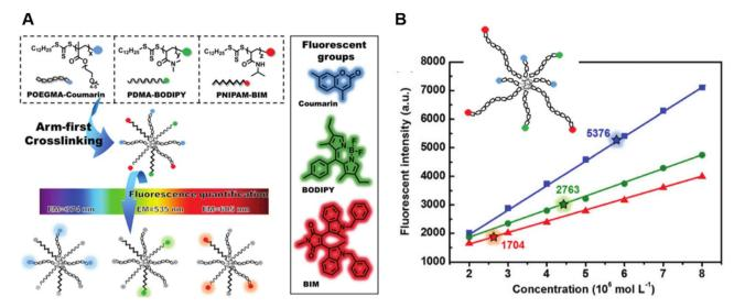
Fig. 6 (A) Illustration of the arm-first approach for the synthesis of miktoarm star polymers bearing different fluorescent end-groups. (B) Linear fits of fluorescence intensities of mikto-star arms with the same monomeric units but different molecular weights, as shown in the inset, to quantify miktoarm star composition. Reproduced from ref. 184 with permission from The Royal Society of Chemistry, copyright 2022.
