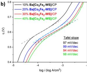
Fig. 5 (a) Rotating disk electrode linear sweep voltammetry (RDE-LSV) of BalCo<sub>2</sub>Fe<sub>2</sub>-WSI/CP electrodes at increasing catalyst loading in the CP blend. (b) Tafel plots obtained from the RDE-LSV data. The dashed lines indicate the Tafel regions. The experiments were conducted in a single-cell using a pH 7.2, 50 mM KP; buffer and KNO<sub>3</sub> (1 M) as electrolyte. The scan rate was 1 mV  $\rm s^{-1}$  at a rotation speed of 1600 rpm.
