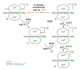
Fig. 10 Schematic representation of the double protonation of  $[Co_2^{II}(H_2O)_2Co^{II}W^{VI}(Co^{II}W_9O_{34})_2]^{12-}$  (A,  $Co_3W$ -WS) and following PCET events, as well as direct ET events. Protonation energies in eV, computed potentials for PCET and ET in V vs. NHE at pH = 7.
