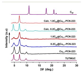
Fig. 2 PXRD data for  $Cu_{0.1}$ -PCN-223 and the  $C_{60}$ @ $Cu_{0.1}$ -PCN-223 composites vs. PXRD data for PCN-223 simulated from the single crystal diffraction data (Cambridge Crystallographic Data Centre (CCDC) code: TUTWUC) and two fulleretic composites optimized in this study (please see Section 2.2).
