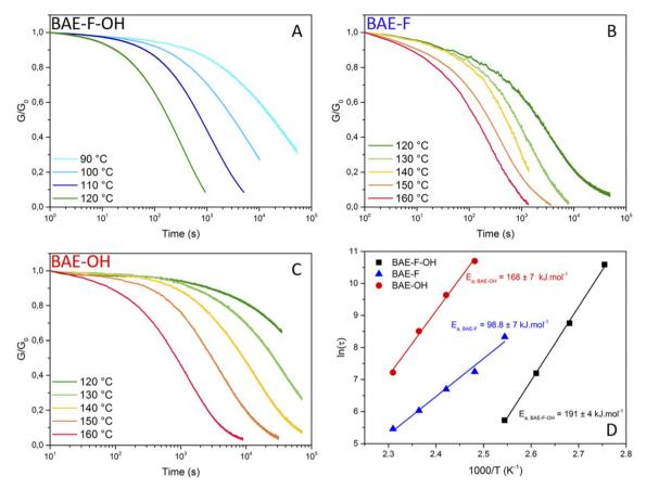
Fig. 4 Normalized stress-relaxation curves at different temperatures for a 1% strain (A) for BAE-F-OH, (B) for BAE-F and (C) for BAE-O. (D) Fitting of the relaxation time (τ) vs. temperature data by the Arrhenius equation for BAE-F-OH (black squares), BAE-F (blue triangle) and BAE-OH (red circles).
