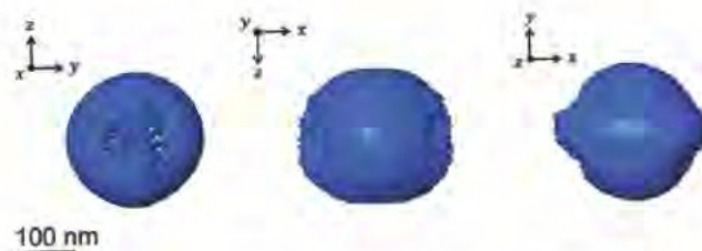
Fig. 5 Visualization of the 3D reconstruction. In the yz plane a spherical shape is observed, while in the zx and xy planes the reconstruction is elongated along the direction of the missing wedge
