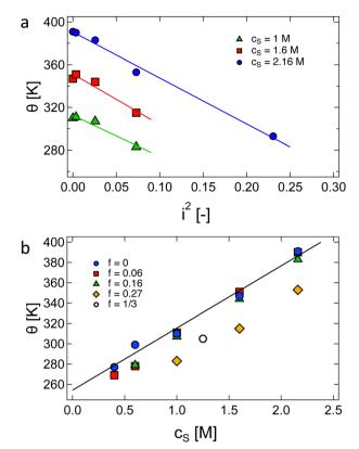
Fig. 4 Dependence of  $\theta$  temperature of polyacrylic acid in aqueous NaCl solutions as a function of (a) the degree of ionisation (i²) squared and (b) the concentration of added salt  $c_s$ . Data are from ref. 192, except for the hollow circle which is from Flory and Osterheld. 195
