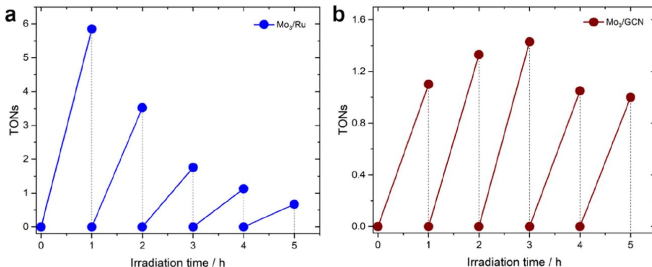
Fig. 5 Long-term HER profiles (in H<sub>2</sub>A) of (a) Mo<sub>3</sub>/Ru system and (b) Mo<sub>3</sub>/GCN system. TONS for the Mo<sub>3</sub>/GCN system were calculated based on real loadings of [Mo<sub>3</sub>S<sub>13</sub>]<sup>2-</sup> clusters on GCN mentioned in Table 1. The experiments were conducted using an LED 445 nm lamp (see Methods section 4.3 for more details).
