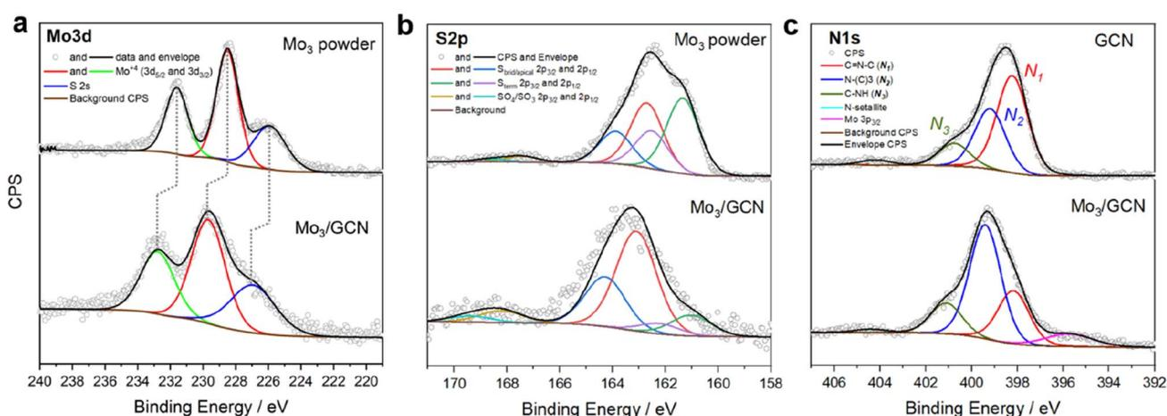
Fig. 3 XPS spectra of the Mo<sub>3</sub>/GCN cluster. The [Mo<sub>3</sub>S<sub>13</sub>]<sup>2-</sup> clusters before (Mo<sub>3</sub> powder) and after (Mo<sub>3</sub>/GCN) attachment to the GCN surface, (a) Mo 3d, (b) S 2p, and (c) N 1s (N<sub>1</sub>: pyridinic nitrogen; N<sub>2</sub>: quaternary nitrogen; N<sub>3</sub>: secondary amine), with corresponding fits.
