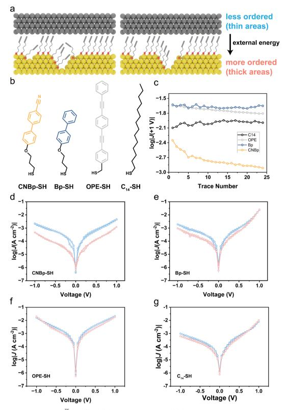
Fig. 1 (a) Schematic illustration of Au<sup>TS</sup>-SAM//Ga<sub>2</sub>O<sub>3</sub>/EGaIn molecular junctions. (b) Chemical structures of the thiol precursors. (c) Plots of tunneling current  $\log |J(+1.0 \text{ V})|$  versus sweep number for the molecular junctions. (d-g)  $\log |J(V)|$  plots for the molecular junctions at the first sweep and last sweep.
