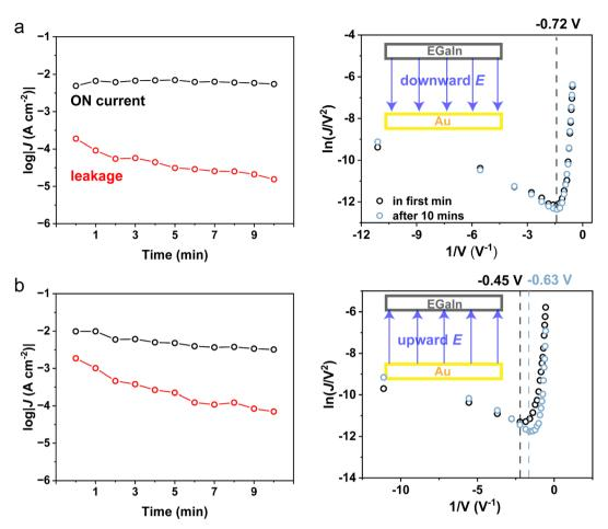
Fig. 4 Plots of  $\log |J(\pm 1.8 \text{ V})|$  measured every 1 min when applying (a) downward and (b) upward  $\vec{E}$  on Au-S-B1-Fc//Ga<sub>2</sub>O<sub>3</sub>/EGaIn junctions and corresponding transition voltage spectrum. The dashed lines correspond to the transition voltage, reflecting the tunneling barrier height in the SAMs//Ga<sub>2</sub>O<sub>3</sub> interface.
