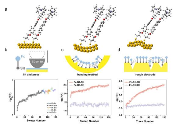
Fig. 6 (a) Simple CPK models of Au–S–B1–Fc dimer under different substrates. (b) Successful enhancement of rectification on molecular diodes of  $Au^{TS}$ –S–B1–Fc// $Ga_2O_3$ /EGaIn in 100 sweeps (black scatters), followed by breaking and forming junctions at the same place five times (colored scatters). (c) Enhancement of log(RR) on bending testbed with bending radius of 17.0 mm. (d) Enhancement of log(RR) can be observed on rough electrodes  $Au^{DE}$  (RMS = 1.0 nm) as well.
