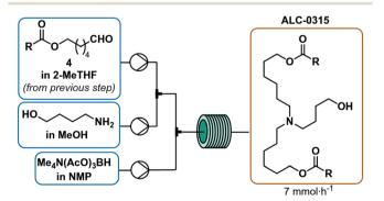
Scheme 5 Continuous reductive amination process for the synthesis of the target tertiary amine 1. Reaction conditions: aldehyde 4 in 2-MeTHF (3 equiv., 0.55 M), 4-aminobutanol in methanol (1 equiv., 0.2 M) and tetramethylammonium triacetoxyborohydride in NMP (3 equiv., 0.45 M) are reacted at room temperature for 16 min.
