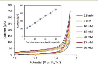
Fig. 3 Inline cyclic voltammetry measurements of a series of solutions 1-phenylethanol (1a) with variable concentrations flowing through the system. Flow rate: 70  $\mu$ L min<sup>-1</sup>.
