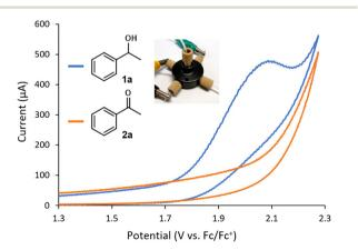
Fig. 2 Cyclic voltammograms of 1a and 2a measured in flow mode using the cell. Conditions: 8 mM substrate in MeCN with 0.1 M Et<sub>4</sub>NBF<sub>4</sub>, flow rate = 70  $\mu$ L min<sup>-1</sup>, scan rate = 0.4 V s<sup>-1</sup>.
