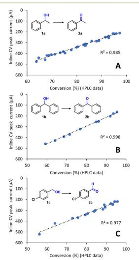
Fig. 5 Comparison of the inline CV response with offline HPLC conversion data for the preparative-scale oxidation of (A) 1a, (B) 1b and (C) 1c. The setup shown in Fig. 4 was used in all cases. The  $R^2$  for linear regression is also shown.
