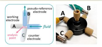
Fig. 1 Schematic view of the flow cell for cyclic voltammetry (left) and photograph of the device (right). A: Pt wire; B: Ag wire; C: Pt wire.
