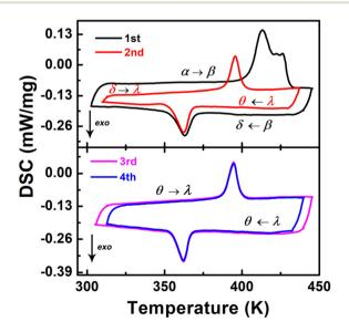
Fig. 3 DSC in several cycles upon heating and cooling for [4,4-DFPD]<sub>2</sub>PbBr<sub>4</sub>. The arrow of exo indicates the exothermic direction.
