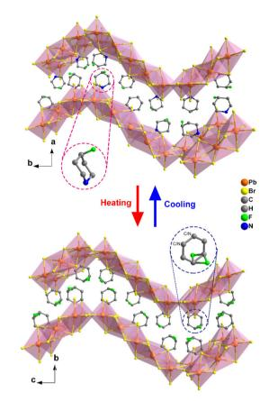
Fig. 2 Comparison of the packing structures of [4-FPD]<sub>6</sub>Pb<sub>5</sub>Br<sub>16</sub> at 299 K (upper) and 440 K (lower). All the hydrogen atoms were omitted for clarity.
