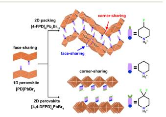
Scheme 1 Structural schematic diagram of [PD]PbBr<sub>3</sub>, [4-FPD]<sub>6</sub>Pb<sub>5</sub>Br<sub>16</sub>, and [4,4-DFPD]<sub>2</sub>PbBr<sub>4</sub>.
