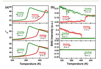
Fig. 5 Temperature-dependence of  $\varepsilon'$  (a) and SHG signal intensity (b) of the [4,4-DFPD]<sub>2</sub>PbBr<sub>4</sub> powder sample measured in three successive heating-cooling cycles.
