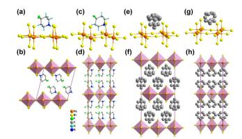
Fig. 4 Crystal structures and packing of  $[4,4-DFPD]_2PbBr_4$ .  $\alpha$  phase at 293 K along the b-axis (a and b);  $\delta$  phase at 293 K along the c-axis (c and d);  $\lambda$  phase at 420 K along the a-axis (e and f) and  $\theta$  phase at 293 K along the a-axis (g and h), respectively. All the H atoms were omitted for clarity.
