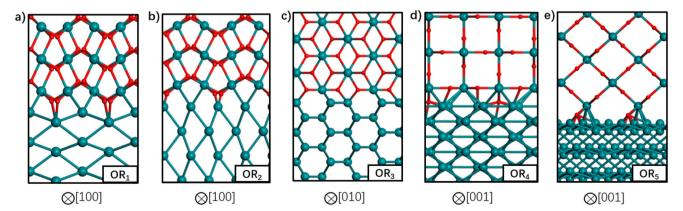
Fig. 8 Atomic structures of the five most stable  $Ru-RuO_2$  interfaces with different orientation relationships (OR) in order of increasing interfacial energy from (a) to (e). Ru atoms are depicted by the green balls and O atoms by the red balls. The crystallographic direction in  $RuO_2$  bulk is indicated below each interface. This figure has been reprinted from ref. 120 with permission from the American Chemical Society, copyright 2021.
