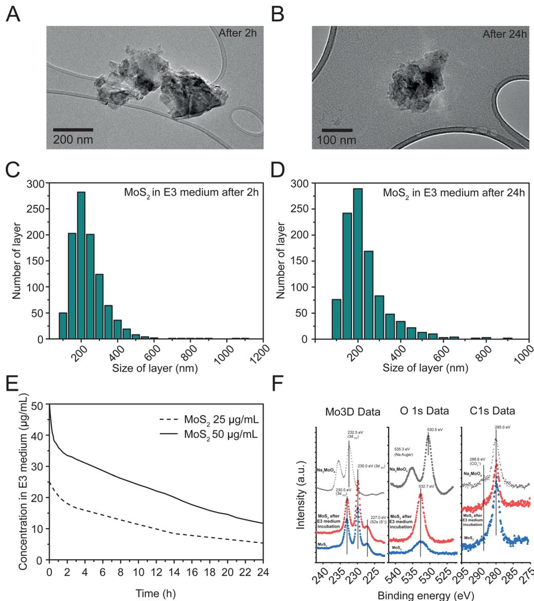
**Fig. 1** Characterization of exfoliated MoS<sub>2</sub>. (A) HRTEM images after 2 hours and (B) 24 hours and corresponding layer size distributions in E3 medium after 2 hours (C) and 24 hours (D). (E) Colloidal stability of MoS<sub>2</sub> in zebrafish E3 medium at 25 and 50 µg mL<sup>-1</sup> during 24 h. (F) Signals from XPS analyses before (blue traces) and after 24 hours exposure to E3 medium (red traces). Molybdate salt (black traces) was used as reference control.
