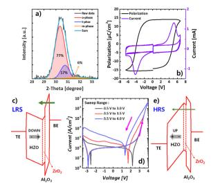
**Fig. 6** GIXRD spectrum of the 7-nm-thick ferroelectric film: deconvolution peaks and the relative ratio of the o-phase, t-phase, and m-phase in the HZO film (a). Polarization switching current by PUND measurement and the corresponding polarization–voltage (*P–V*) curve (b) and double sweep *IV* characteristics with various sweep ranges (d). Energy band diagram for LRS (c) and HRS (e) of FTJ.
