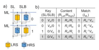
**Fig. 1** (a) Schematic of the common two resistance-based CAM utilizing passive components. ML, SL, and SLB denote the match line, search line, and complementary search line, respectively. (b) Encoding of a 1-bit key using SL and SLB and 1-bit content using left and right resistors ( $R_{\text{left}}$  and  $R_{\text{right}}$ ).  $V_{\text{H}}$  is a pull-up voltage. Matching result is obtained with minimum value of ML current ( $I_{\text{ML}}$ ).
