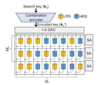
Fig. 2 Schematic of N-CECAM (N = 4). The search key  $\mathbf{k}_{\rm b}$  is encoded into a 2N-long binary array  $\mathbf{k}'_{\rm b}$  by the combination encoder. Each bit of the encoded key represents the corresponding voltage at search lines (low voltage for 0s and high voltage for 1s). Matching search is obtained at the lowest matching current.
