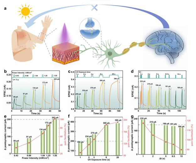
Fig. 4 (a) Schematic diagram of the device detecting, recognizing, and self-protecting against UV stimuli. (b) EPSC and (e)  $\Delta$ PSC and pain facilitation under different UV irradiation intensities (320 nm, pulse width of 1 s). (c) EPSC and (f)  $\Delta$ PSC and pain facilitation under different UV irradiation intervals (320 nm, 1.25 mW cm<sup>-2</sup>). (d) EPSC and (g)  $\Delta$ PSC and pain facilitation under different UV irradiation intervals (320 nm, 1.25 mW cm<sup>-2</sup>).
