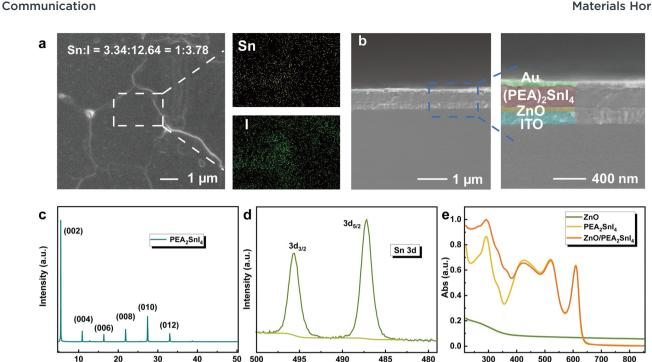
Fig. 2 (a) Top-view SEM image of PEA<sub>2</sub>SnI<sub>4</sub> and mapping images for the corresponding elements (Sn and I). (b) Cross-sectional image of the PEA<sub>2</sub>SnI<sub>4</sub>/ ZnO device. (c) XRD pattern of PEA<sub>2</sub>SnI<sub>4</sub> film. (d) XPS spectra of PEA<sub>2</sub>SnI<sub>4</sub>: Sn 3d. (e) Absorption spectrum of ZnO, PEA<sub>2</sub>SnI<sub>4</sub>, and the PEA<sub>2</sub>SnI<sub>4</sub>/ZnO films.
