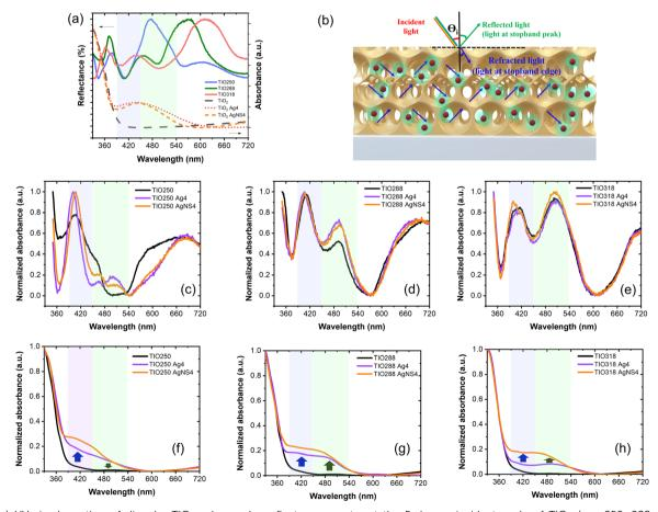
Fig. 6 (a) UV-vis absorption of disorder TIO and specular reflectance spectra at the 5-degree incident angle of TIOx (x = 250, 288, and 318). (b) Schematic of the distribution of the Ag NPs (red) and the absorbed light scattered by the IO structure. Normalized specular absorbance spectra at the 5-degree incident angle and transparency spectra of (c) and (f) TIO250, (d) and (g) TIO288, and (e) and (h) TIO318 deposited Ag NPs.
