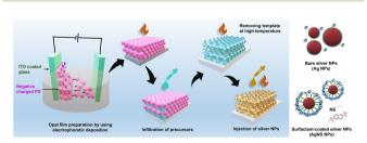
Fig. 1 Schematic of the synthesis process of the TiO<sub>2</sub> IO films, deposition of the Ag and NS-modified Ag NPs inside the IO walls, and different Ag NP structures
