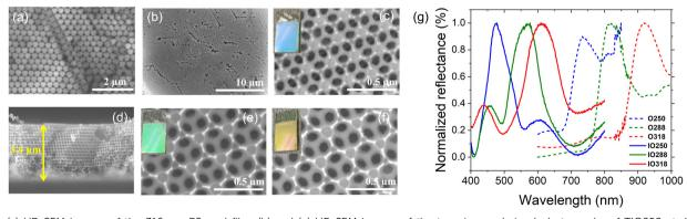
Fig. 2 (a) HR-SEM images of the 316 nm PS opal film, (b) and (c) HR-SEM images of the top view and visual photographs of TIO250 at different magnifications, and (d) HR-SEM images of the cross-section view of TIO250. HR-SEM images of the top view of (e) TIO288 and (f) TIO318. (g) Specular reflectance spectra at the 5-degree incident angle of the PS opal (O) film and TIO films prepared using different PS bead sizes.
