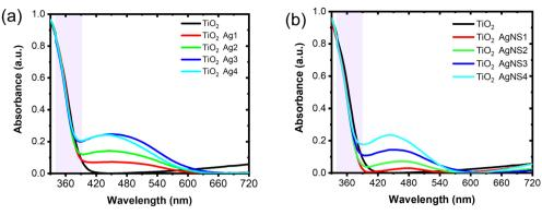
Fig. 4 UV-vis absorption spectra of (a) disorder Ag-deposited TiO<sub>2</sub> IO, and (b) disorder AgNS-deposited TiO<sub>2</sub> IO.
