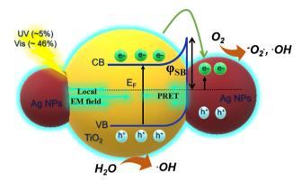
Fig. 9 Scheme of the effect of LSPR and slow photon effect on the generation of electron/hole pairs on Ag-deposited TiO2 by absorbing
