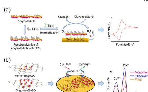
Fig. 4 Application of amyloid-based fibrils in sensors: (a) immobilization of glucose oxidase for the development of the electrochemical glucose biosensor and (b) amyloid-rGO composite (ArGOC) based amperometric sensor for detection of heavy metals.
