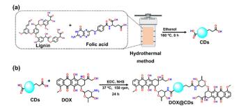
Scheme 2 Schematic illustration of the carbon dots (CDs) (a) synthesis from lignin and folic acid as a coating via a hydrothermal method and (b) the conjugation of doxorubicin (DOX) on CDs (DOX@CDs).
