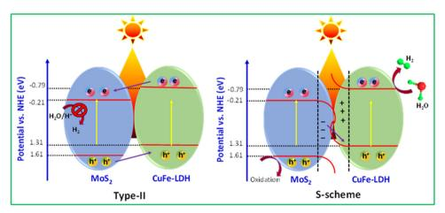
Fig. 8 Mechanism of photocatalytic  $H_2$  creation from the CuFe-LDH/MoS $_2$  system
