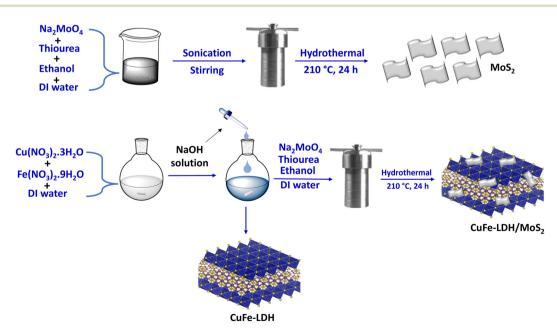
Scheme 1 Synthetic procedure of MoS<sub>2</sub>, CuFe-LDH, and the CuFe-LDH/MoS<sub>2</sub> nanocomposite.
