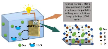
The application of MOFs in sodium ion batteries. 130
