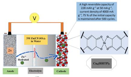
Fig. 9 The application of MOFs in zinc ion batteries. 139
