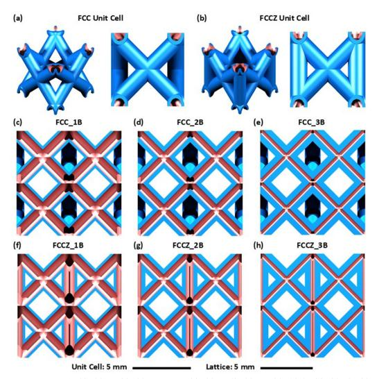
Fig. 1 Hollow-strut lattice models for (a) FCC and (b) FCCZ topologies. (c) FCC\_1B, (f) FCCZ\_1B, (d) FCCZ\_2B, (g) FCCZ\_2B, (e) FCCZ\_3B, and (h) FCCZ\_3B. The blue coloration indicates hollow-strut walls while the light red coloration characterizes the internal profiles.  $\Delta D$ : wall thickness.
