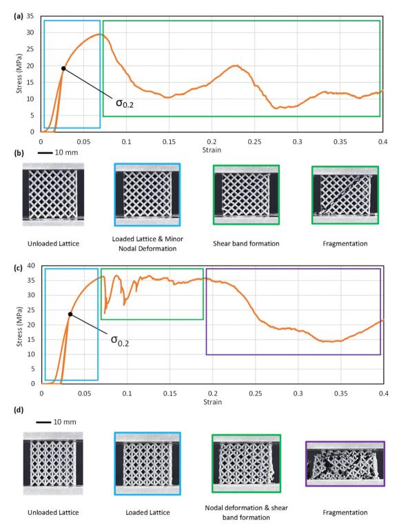
Fig. 9 Failure modes and stress-strain curves. (a) The stress-strain curve for FCC\_2B AlSi10Mg hollow-strut lattices. (b) Photos of lattice specimens corresponding to different deformation stages in (a). (c) The stress-strain curve for FCCZ\_2B AlSi10Mg hollow-strut lattices. (d) Photos of lattice specimens corresponding to different deformation stages in (c).
