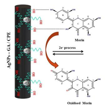
Fig. 11 Schematic representation of the mechanism of the electrochemical oxidation of morin at AgNP-gum Arabic (GA)/CPE (reprinted from ref. 150 with permission from Elsevier).
