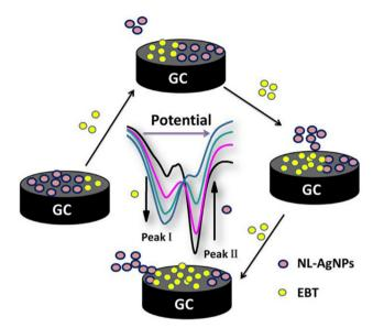
Fig. 15 Schematic representation of the electrochemical displacement of AgNPs by Eriochrome black T (EBT) (reprinted from ref. 166 with permission from Elsevier).
