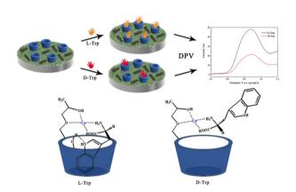
Fig. 7 Schematic representation the of electrochemical chiral recognition of tryptophan isomers (reprinted from ref. 81 with permission from Elsevier).
