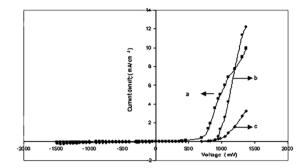
Fig. 7 Current density v/s voltage (a) CdS/polyaniline, (b) CdSe/polyaniline, and (c) CdTe/polyaniline. [Reproduced from ref. 35, with permission from Springer, Copyright 2007.]
