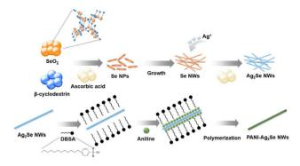
Fig. 11 Synthesis of polyaniline-Ag₂Se nanowires. [Reproduced from ref. 40, with permission from Elsevier, Copyright 2021.]
