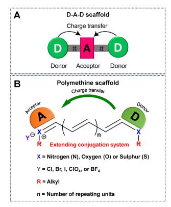
Fig. 2 Schematic representation of a universal scaffold for (A) D-A-D and (B) polymethine based fluorophores.
