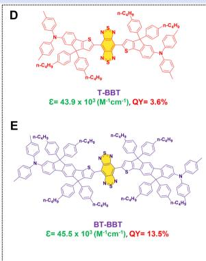
Fig. 11 D-A-D based fluorophores (A-E) with planar and twisted molecular architectures for high QY and high  $\varepsilon$ .
