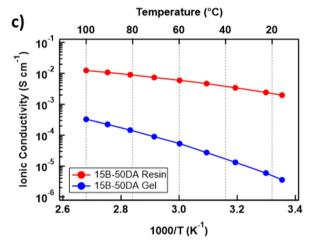
Fig. 2 Characterization of ionic liquid gels. (a) Tensile strength of gels with varying amounts of copolymer. (b) Tensile experiments of formulation 7.5–7.5-BVIM after printing, after being cut and mechanically mended (pushed together), and after being thermally mended at 85 °C. (c) Electrical Impedance Spectroscopy (EIS) data of formulation 7.5–7.5-BVIM as a resin (red) and after printing (blue) over a range of temperatures (20–100 °C).
