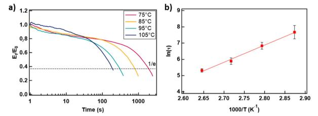
Fig. 3 (a) Stress relaxation of 7.5–7.5-BVIM gels at varying temperatures. Relaxation times ( $\tau$ ) are determined when the normalized modulus reaches 1/e of the initial value. (b) Activation energy ( $E_a$ ) of Diels–Alder bonds in the network was determined from the slope of the natural logarithm of  $\tau$  plotted against 1000/T ( $E_a$  = 84  $\pm$  5 kJ mol<sup>-1</sup>).
