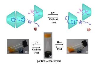
Fig. 47 (a) Mode of inclusion between b-CD and AzoIPS-LiTFSI before and after UV irradiation. (b) Preparation of the supramolecular hydrogel: (a) b-CD/AzoIPS-LiTFSI (3:1), and its disassembly induced by: (b) UV light, and (c) temperature. Reproduced from ref. 226 with permission from Wiley-VCH, Copyright [2018].
