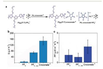
Fig. 54 (a) Structure of the  $P(g_42T-T)$  with croconate<sup>-2</sup>. Thermoelectric parameters of chemically doped and ion exchange P(g<sub>4</sub>2T-T) films. (b) Seeback coefficients (S) and (c) power factors (PF) of P(q<sub>4</sub>2T-T):PF<sub>6</sub><sup>-</sup>, P(q<sub>4</sub>2T-T):PF<sub>6</sub><sup>-</sup>, low, and P(q<sub>4</sub>2T-T): croconate<sup>-2</sup> thin films Reproduced from ref. 234 with permission from Wiley-VCH, Copyright [2023].
