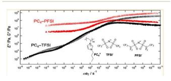
**Fig. 27** Elastic modulus of imidazolium-based polymerized ionic liquids upon introducing large counteranions. Reproduced from ref. 43 with permission from ACS, Copyright [2018].
