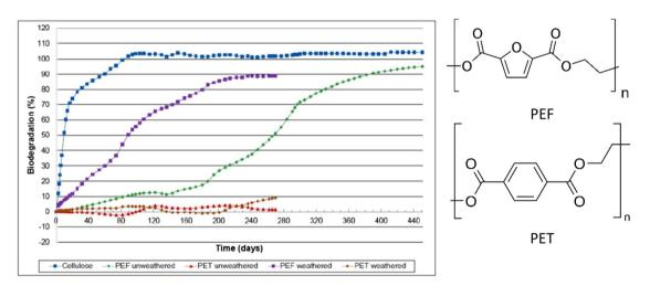
Fig. 8 Biodegradation profiles of weathered and un-weathered PEF, as well as weathered and un-weathered PET and cellulose as a reference material. Biodegradation (%) = amount of polymer converted to  $CO_2$  (up to 450 days) with air/oxygen @ 58 °C in soil. All curves are the averages of three samples.<sup>85</sup>
