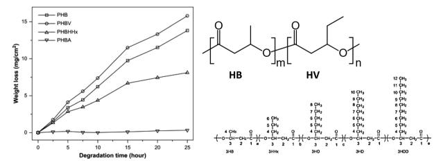
Fig. 18 Enzymatic degradation of PHBV (94%), PHB (75%), PHBHHx (39%) and PHBA (0%) by PHA depolymerase produced by Ralstonia pickettii T1 at 37 °C. Structures of monomers and PHBV (m-HB, n-HV, as an example for copolymers). Reproduced from ref. 100 with permission from Elsevier, copyright 2007.
