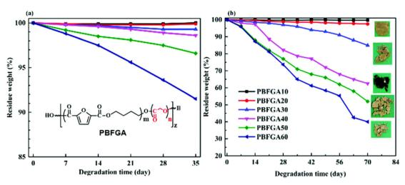
Fig. 9 Weight loss curves of PBFGAs during hydrolysis (a), enzymatic degradation (b) and visual observations of degraded films after 70 d at 37 °C. Note: Scales are not equal for (a) and (b). Reproduced from ref. 86 with permission from the Royal Society of Chemistry, copyright 2019.
