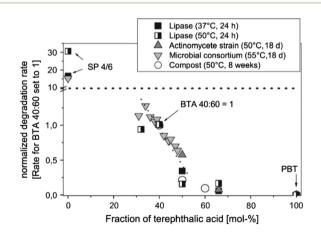
**Fig. 5** Dependence of the degradation rate of aliphatic–aromatic copolyesters (BTA-copolyesters, PBAT) on the content of terephthalic acid in the polymer in different degradation environments. The absolute degradation rates are normalised to the rate for the random copolyesters BTA<sub>random</sub> 40:60. B: 1,4-Butanediol unit; T: terephthalic acid unit; A: adipic acid unit; SP 4/6: poly(butylene adipate) (SP 4/6). Reproduced from ref. 62 with permission from Elsevier, copyright 2005.
