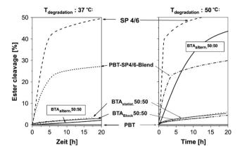
**Fig. 6** Degradation of polyesters of different micro-structure by a lipase from *Pseudomonas* sp. (PsL) at 37 °C and 50 °C in water. Degradation was monitored by titrating the acid groups formed during ester cleavage. B: 1,4-Butanediol unit; T: terephthalic acid unit; A: adipic acid unit; SP 4/6: poly(butylene adipate) (SP 4/6). Reproduced from ref. 62 with permission from Elsevier, copyright 2005.
