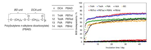
Fig. 13 BOD biodegradation curves of 1,4-butanediol (BD), n-alkylene dicarboxylic acid (DCAs), including tridecanoic diacid (n = 11; TrdA), tetradecanoic diacid (n = 12; TedA), pentadecanoic diacid (n = 13; PdA), and hexadecanoic diacid (n = 14; HdA), and PBADs at 25 °C for 45 days. Reproduced from ref. 92 with permission from Elsevier, copyright 2021.
