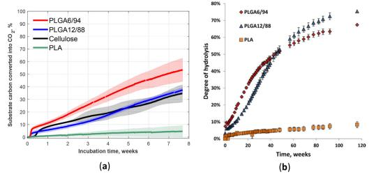
Fig. 17 Fifty-three-day biodegradation curves of PLA, PLGA12/88, PLGA6/94 and cellulose (reference) at 25 °C in soil (a). Mean biodegradation (lines) were plotted. The shaded area represents the standard deviation of replicates. Degree of hydrolysis for PLGA6/94, PLGA12/88 and PLA versus time over 116 weeks at 25 °C in D<sub>2</sub>O (b). The points represent the averages of triplicate experiments, with the error bars representing the standard deviation
