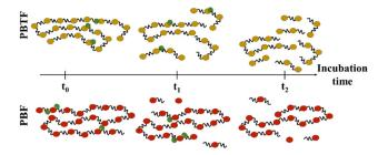
Fig. 4 Enzymatic hydrolysis mechanisms. The endo-wise hydrolysis mechanism for PBTF (top) leads to the release of oligomers, which are subsequently hydrolysed to monomers. In contrast, the exo-wise hydrolysis mechanism for PBF (bottom) leads to the immediate release of monomers. Reproduced from ref. 82 with permission from Elsevier, copyright 2019.
