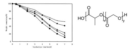
Fig. 16 Weight remaining percentage of (—) PLA, (●) PLGA (85/15), (▲) PLGA (75/25), (●) PLGA (65/35), and (■) PLGA (50/50) microspheres containing human serum albumin incubated in phosphate-buffer saline (154 mM, pH 7.4) at 37 °C. Each point represents the mean of three individual samples of microspheres. Reproduced from ref. 98 with permission from John Wiley & Sons Inc., copyright 2003.
