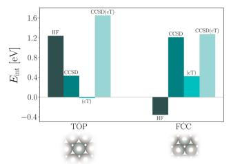
Fig. 2 Bar plot showing energy contributions to the CO interaction energy on the top and fcc hollow site of Pt(111). HF disfavors and favors adsorption on the fcc and top site, respectively. CCSD and (cT) correlation energy contributions are also illustrated. The final estimates of the CO/Pt(111) interaction energies for the fcc and top site are given by the bars labelled CCSD(cT).
