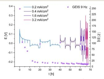
Fig. 5 Voltage traces (E-t) of galvanostatic plating of 1 mA h cm $^{-2}$  Li at increasing current densities between 0.2 and 3.2 mA cm $^{-2}$  in a Li symmetric cell, LP30 electrolyte and GF separator at RT. EIS intensity (purple spheres) measured with GEIS at 9 Hz with 100  $\mu$ A amplitude.
