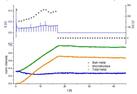
Fig. 8 Operando  $^7$ Li NMR and impedance (GEIS) measured at 8 Hz intensities measured during unidirectional Li plating at 1 mA cm $^{-2}$  in an NMR in situ cylindrical symmetrical Li cell with LP30 electrolyte.
