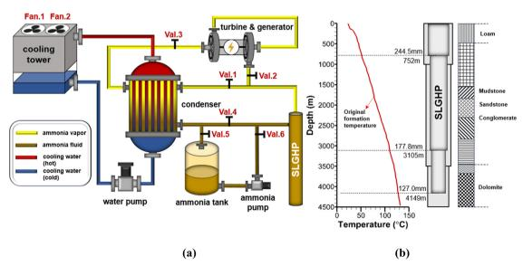
Fig. 2 (a) SLGHP geothermal system constructed in Xiong'an, China; (b) measured temperature in the original geothermal formation, well-borehole configuration after assembly with the SLGHP, and local geological formation.
