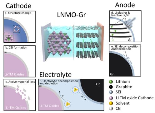
Fig. 1 Schematic of active Li inventory loss in Li transition metal (TM) oxide cathode/Graphite full cells. (a) Cathode structure change; (b) CEI formation; (c) active material loss; (d) Li plating and trapped Li<sub>x</sub>C<sub>6</sub>; (e) SEI formation; (f) electrolyte decomposition.
