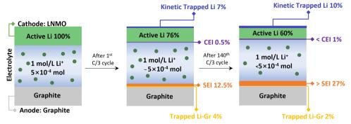
Schematic of Li inventory evolution in the LNMO-graphite pouch cell system with Gen2 electrolyte
