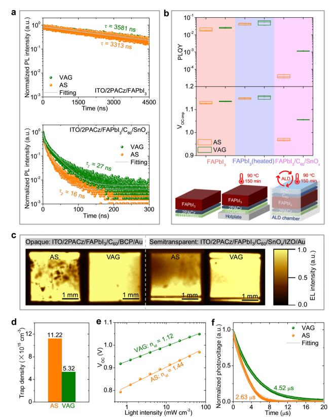
Fig. 4 Characteristics of non-radiative recombination for middle sub-cell. (a) TRPLs and (b) PLQYs for ITO/2PACz/FAPbI<sub>3</sub> and ITO/2PACz/FAPbI<sub>3</sub>/C<sub>60</sub>/ SnO<sub>x</sub> stacks. (c) EL imaging of opaque and semitransparent single-junction FAPbI3-based devices. (d) Trap density obtained from the SCLC method, (e) light intensity dependence of the V<sub>OC</sub>, and (f) normalized transient photovoltage decay of semitransparent FAPbl<sub>3</sub>-based devices.
