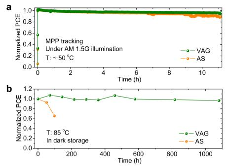
Fig. 5 Durability of perovskite-perovskite-Si MTJSCs. Evolution of normalized PCEs of perovskite-perovskite-Si MTJSCs (a) under continuous AM 1.5G illumination at  $\sim 50$  °C for MPP tracking and (b) in dark storage at 85 °C. All devices without encapsulation were tested in an N<sub>2</sub>-filled glovebox.
