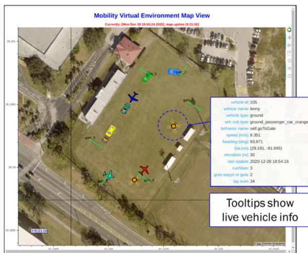
Fig. 7 MoVE 2D map display with icons of ground vehicles, fixed-wing aircraft, multirotor aircraft, and pedestrians. Fixed-wing and multirotor are different subtypes of the same aerial type.
