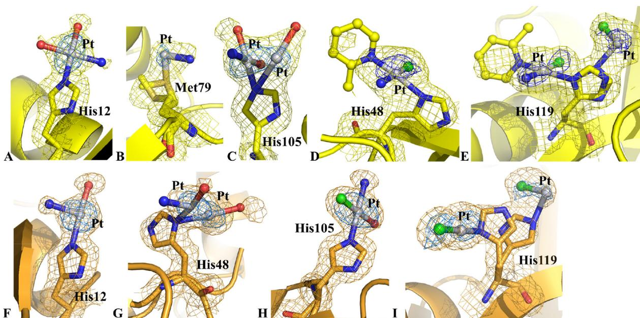
**Fig. 6** Picoplantin derivative binding sites in RNase A structure **D**. Pt fragments bind the side chains of His12 (panels A and F), His48 (panels D and G), His105 (panels C and H) and His119 (panels E and I) of both protein chains of the a.u., and the side chain of Met79 in chain 2 (panel B). 2Fo–Fc is contoured at 1.0  $\sigma$  level. Chain 1 is in yellow, chain 2 in bright orange. Anomalous difference electron density map is reported at 4.0  $\sigma$  level in blue.
