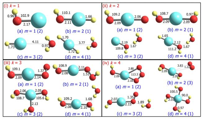
Fig. 2 Ground state structures of  $AgO_kH_m^-$ , where k, m = 1-4, optimized at the CCSD level. Bond lengths and angles are given in Angstroms and degrees, respectively. The spin multiplicity (2S + 1) of the  $AgO_kH_m^-$  clusters is provided in the parentheses.
