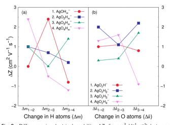
Fig. 9 Difference in electrical mobility,  $\Delta Z$ , (in cm<sup>2</sup> V<sup>-1</sup> s<sup>-1</sup>) between (a)  $AgO_kH_{m-1}^-$  and  $AgO_kH_m^-$  clusters for k=1-4, and m=2-4; (b)  $AgO_{k-1}H_m^-$  and  $AgO_kH_m^-$  clusters for k=2-4, and m=1-4. Z values of  $AgO_kH_m^-$  clusters have been calculated by the TM in helium carrier gas.
