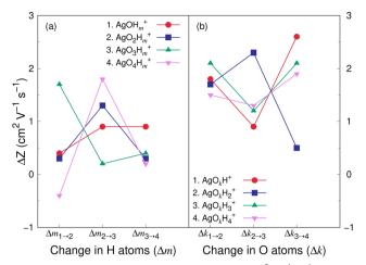
Fig. 8 Difference in electrical mobility,  $\Delta Z$ , (in cm<sup>2</sup> V<sup>-1</sup> s<sup>-1</sup>) between (a)  $AgO_kH_{m-1}^+$  and  $AgO_kH_m^+$  clusters for k=1-4, and m=2-4; (b)  $AgO_{k-1}H_m^+$  and  $AgO_kH_m^+$  clusters for k=2-4, and m=1-4. Z values of  $AgO_kH_m^+$  clusters have been calculated by the TM in helium carrier gas.
