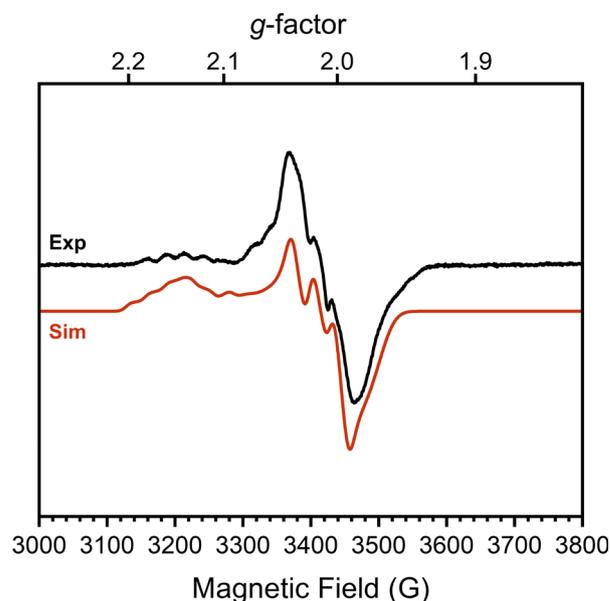
Fig. 2 X-band EPR spectrum (black) and simulated spectrum (red) of a 15 mM solution of **1** (dimer) in toluene at 25 K. Conditions: MW frequency, 9.63 GHz; MW power, 2.0 mW. Simulation parameters:  $g_{x,y,z} = 2.143, 2.015, 1.983$ ; <sup>59</sup>Co  $A_{x,y,z} = 37.85, 7.06, 22.66$  MHz; <sup>14</sup>N  $A_{x,y,z} = 85.39, 87.94, 22.66$  MHz; HStrain<sub>x,y,z</sub> = 41.7975, 32.2248, 100.
