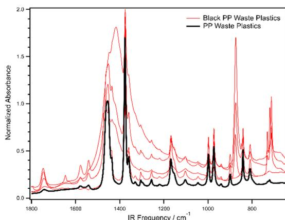
Fig. 5 Polypropylene waste plastic with zero carbon black content (black). Black-colored polypropylene waste plastics (red). Spectra were normalized to the  $2916\text{ cm}^{-1}$  asymmetric methylene stretch.
